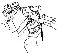
Fig. 14 Cutting the wire
